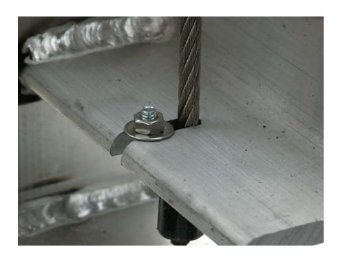
19: Loosen the winch cable retainer located on the winch drum. The winch corner ('Bed A') will have an unfinished cable end. Feed this end up into the winch hub as shown. Note the direction of the cable. Thread through the hole until it is flush with the exit hole. Tighten the set screws.
