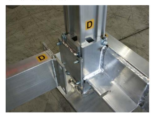
5: While holding the Corner Post 'A' vertical, insert Side Beam 'A', into channel, until the Corner Post is flush with the bottom of the Side Beam Channels. Loosen the screws from the previous step and snug over the channel slots as shown.
