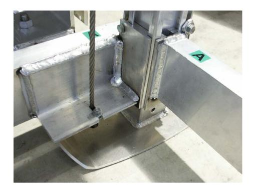
17: Attach the (5) upper cables as shown. The Horizontal Brace side will have (4)  $\frac{1}{2}$ " washes to run the cables through. You may want to lift the bed slightly to facilitate this step. Screw the  $\frac{1}{2}$ -13 nuts onto the screw ends. Level the bed, and snug the screws without over tightening. Too tight and the Bed will tilt down toward the winch, too loose and the Bed will tilt up toward the winch. Jam the second  $\frac{1}{2}$ -13 hex nut on the screw.
