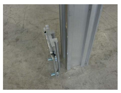
These Beam Insert Plates will attach to the ends of Beam AB and Beam CD, so slide them up the corresponding Corner Posts first. Use the screw from the beginning of this step to tighten these (4) Beam Insert Plates as shown below.
