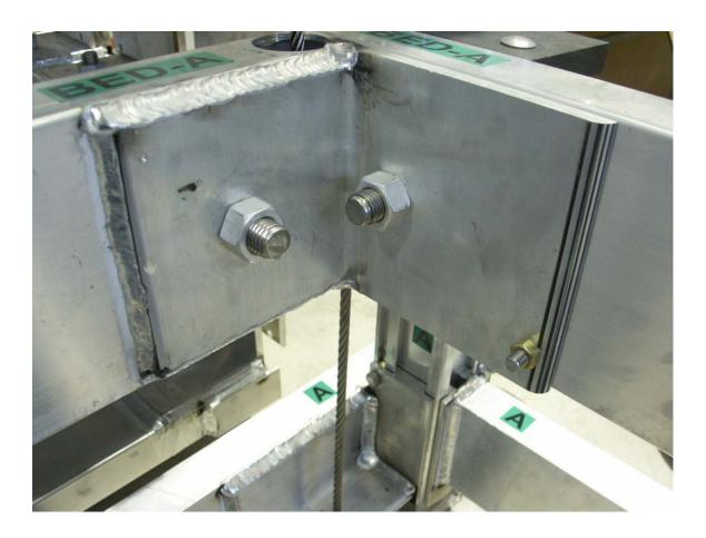
15: After the <sup>3</sup>/<sub>4</sub>-10 screws and the 3/8-16 screws are tightened, rotate the Bed assembly to the left, counter-clockwise into position on top of the wood blocks.
